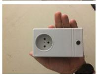
Quantimetrica's SmartPlug monitors speech presence in the vicinity (and as a result human presence) and can operated switch attached mains devices off after a period of inactivity. As a result, devices that have been left on and unattended will switch off automatically. This not only saves energy but prevents potential domestic fires from certain appliances.
